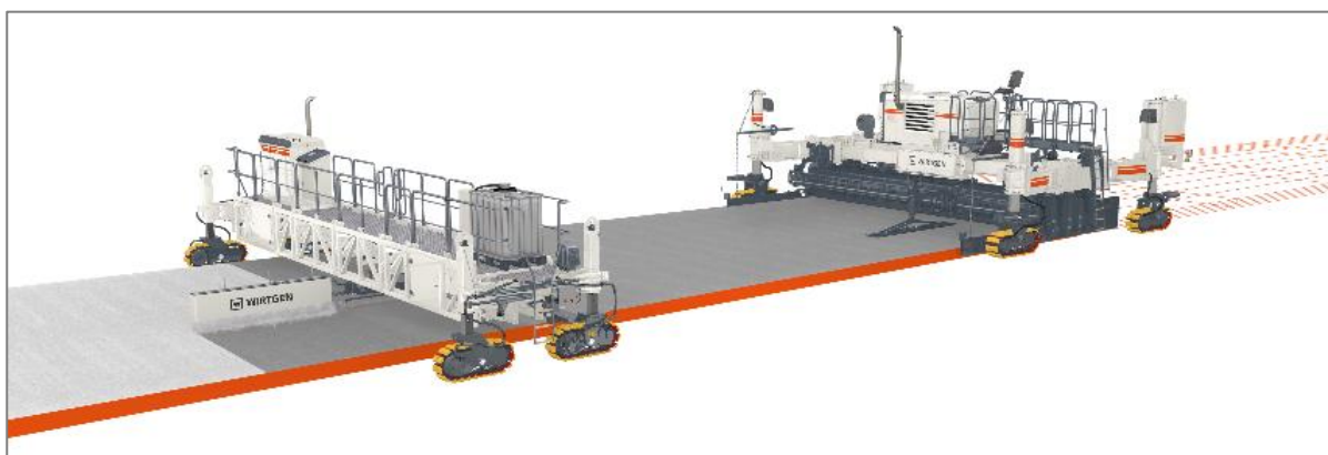
Figure 24: Typical slip-form concrete paving machine operation (from Wirtgen)
